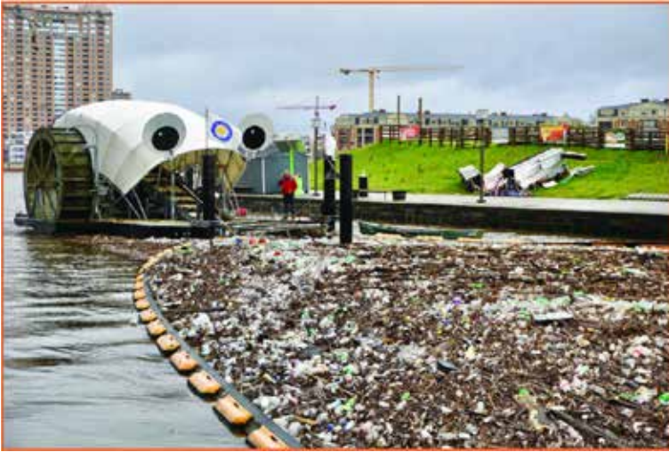
Mr. Trash Wheel gobbles trash floating down the Jones Falls River, protecting both the Baltimore, MD, harbor and the ocean beyond. Photo credit: Waterfront Partnership of Baltimore
